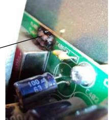
Example for correct mounting resistor with long leg for better cooling / air circulation
